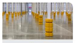
Shock-absorbing assembly installs securely, cushions columns, equipment & drivers during impacts. Column Guard was installed on a fabricated square vertical steel column and impacted with a 500-lb [227 kg] pendulum raised 1.8-ft [0.55 m] from the point of impact to provide an impact energy of 900 ft-lbs. [1222.5 Nm].
