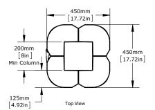
Column Guard Materials: HDPE shell Column Guard, 25mm ratchet and strap system
